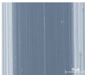
SEM Grade 2 c.p. titanium turned surface. 500 x magnification.
