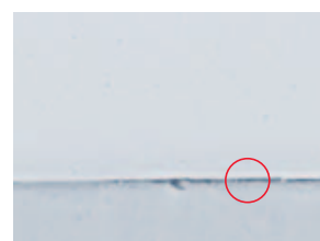
NobelReplace™ Tapered Groovy RP Implant and NobelProcera™ Abutment Zirconia. Scanning electron microscope (SEM) images of abutment/implant interface (precision of fit <math><0.5\mu\text{m}</math>).
