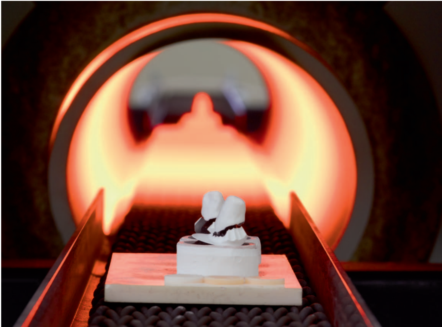
Pre-sintering phase of NobelProcera Alumina Crown coping production.
